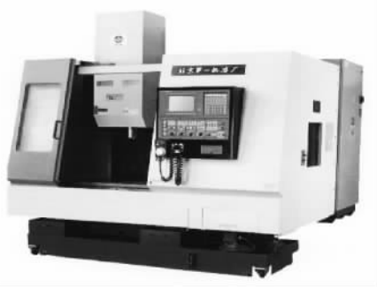
Figure 2-1 A vertical machining center 立式加工中心
