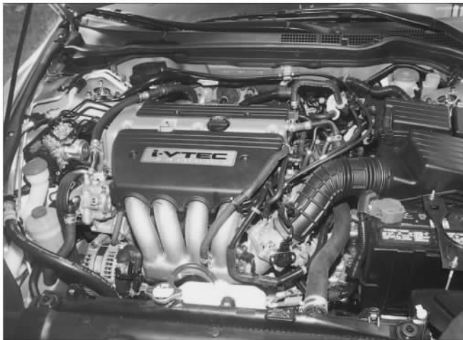
Fig. 2-1 Honda's new 2003 engine is a 2.4 L four that's rotated 180° so the intake is on the front side of the transverse engine and the accessory belt drive is on the passenger side. The distributor is gone.
