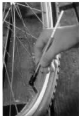
▼ Figure 10.3 A tire pressure gauge is used to measure the extent to which the pressure of the enclosed air exceeds atmospheric pressure.
