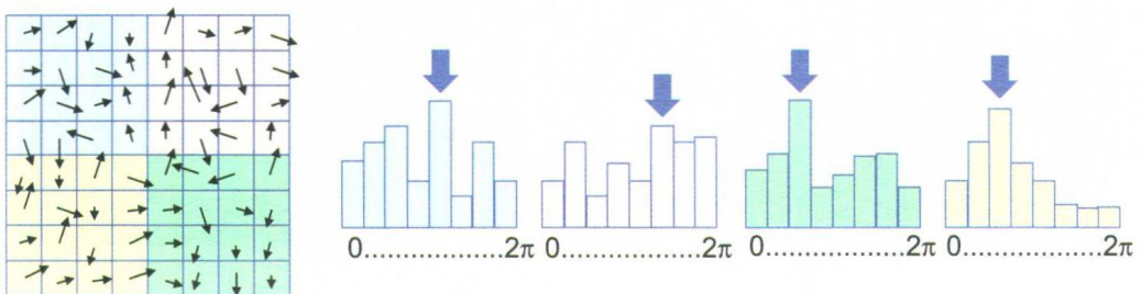
Figure 4.11 SIFT determines gradient vectors for every pixel of the (here: 8 \times 8 ) image patch (left). A (here: 2 \times 2 ) descriptor array with (here: 8-bin) histograms relating cumulative gradient vector magnitude to gradient orientation is built (right). In this example, the descriptor has 2 \times 2 \times 8 = 32 dimensions.
