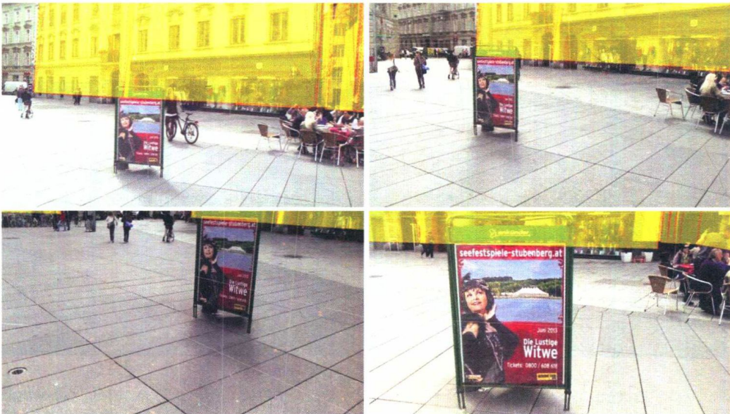
Figure 4.35 This SLAM sequence starts with tracking a facade (overlaid in yellow), for which a global pose has been determined by a server. The images in the bottom row cannot continue tracking with information known to the server; the poster in the foreground, which has been incorporated into the SLAM map, is used for tracking instead. Courtesy of Jonathan Ventura and Clemens Arth.
