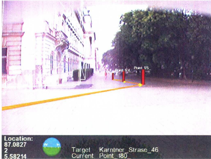
Figure 11.1 The Signpost system lets an outdoor AR user follow a route consisting of waypoints (red cylinders). Courtesy of Gerhard Reitmayr.
