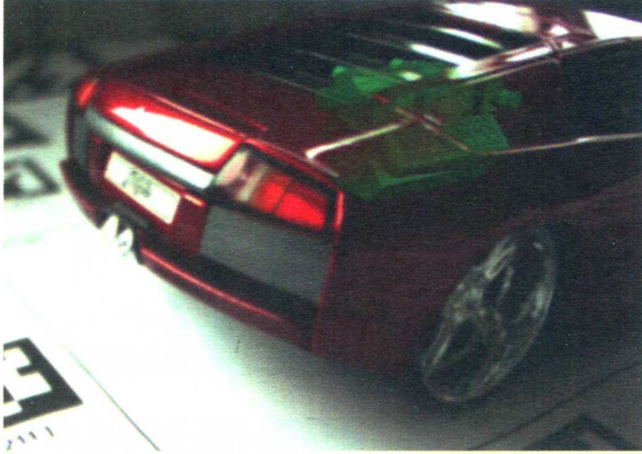
Figure 7.13 In this example, the body of a real car is the occluder for a virtual engine. After extracting contours as important shape hints, a 2D distance transform is applied to make the occluder seem more solid. Courtesy of Denis Kalkofen.
