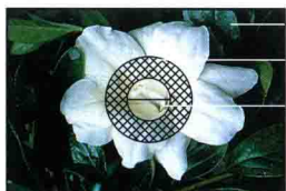
磨砂玻璃 Ground glass 微棱镜 Microprism 裂像 Split image
