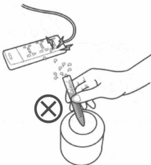
Figure 1.2 Precautions for electrical safety during preparing reagents
