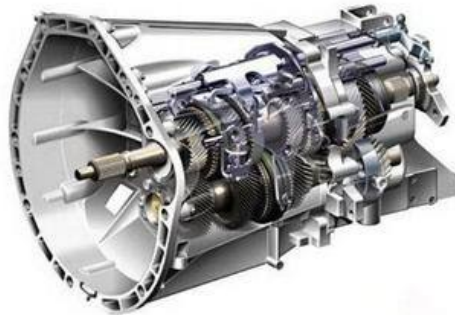
Fig.1.5 Schematic Diagram of MR515B03 Transmission Structure
