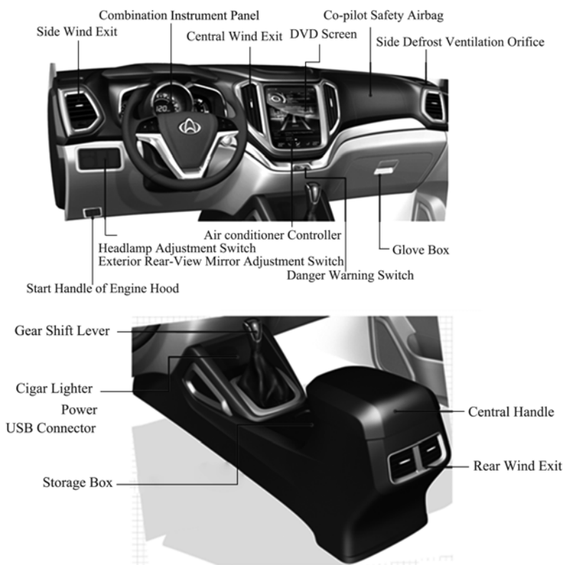
Fig.1.8 Schematic Diagram of CX70 Instrument Panel and Auxiliary Fascia Console
