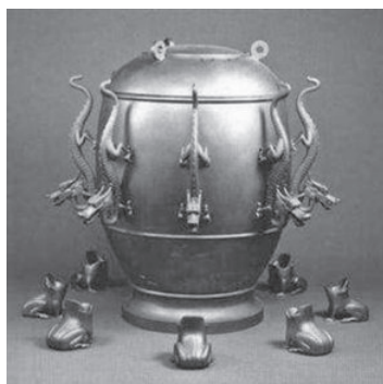
The seismograph invented by Zhang Heng
