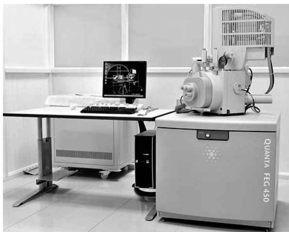
Fig. 1-2 QUANTA FEG450 SEM equipped with a field emission gun
