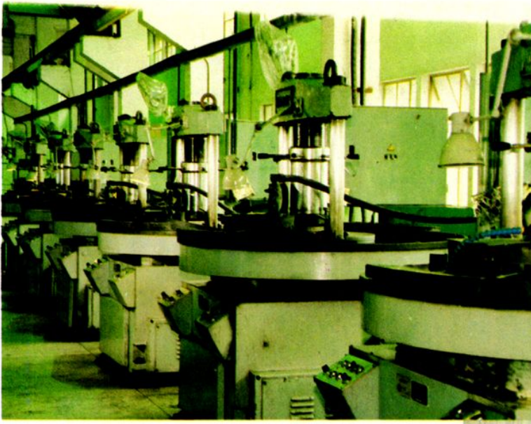
3M4730B 型鋼球精研機
