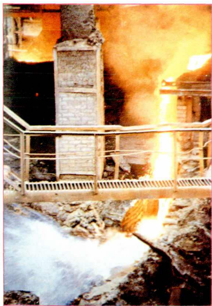
◀ 涟源钢铁厂在国内首创的水力运渣新工艺
