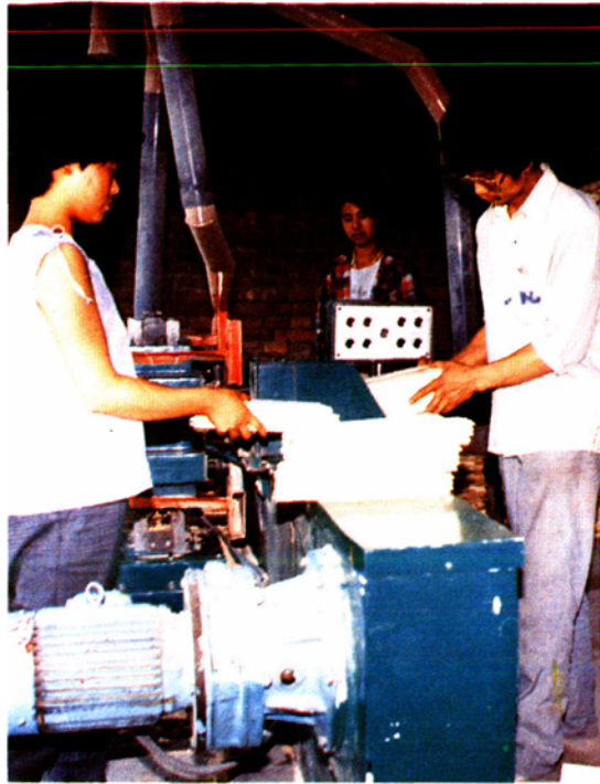
地板塊加工 Wood scraps-composed floor processing
