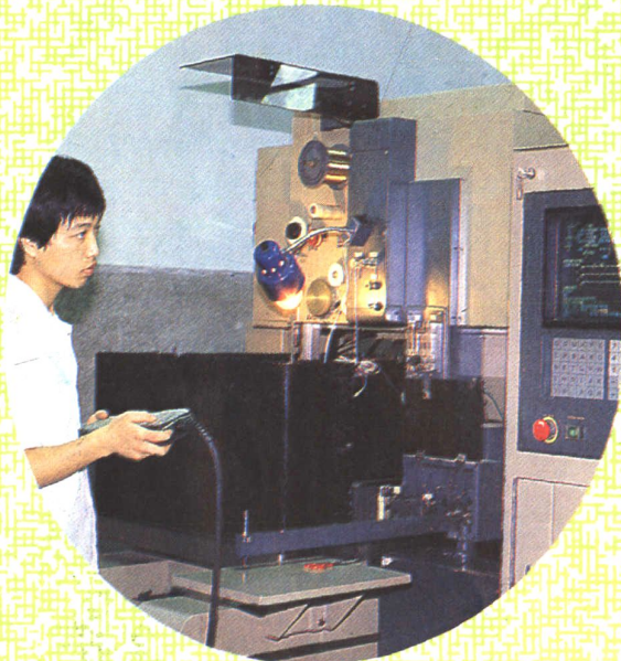
模具生產綫工人在進行模具綫切割 The worker is making dies on numerical control wire cutting machine.
