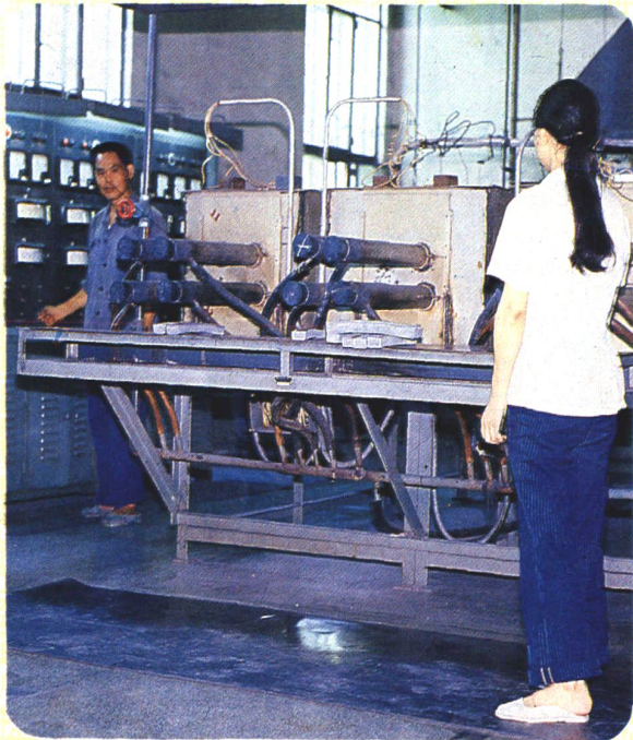
鎢鉬絲生產綫工人在製作材料 Workers on the tungsten and molybdenum wire production line are making billets.
