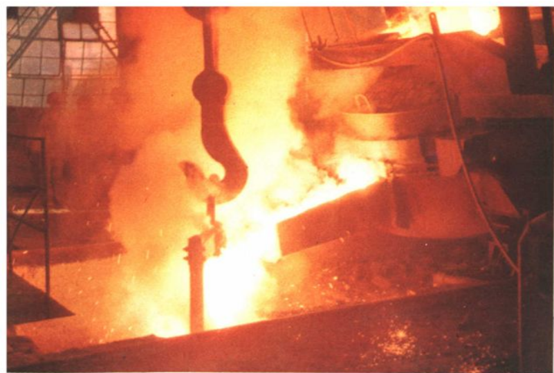
◁1.5吨电弧炉出钢
