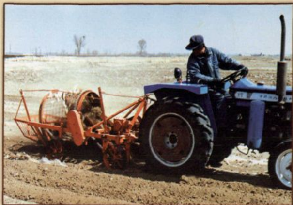
1MC-70型地膜回收起茬机在田间回收地膜和玉米根茬
