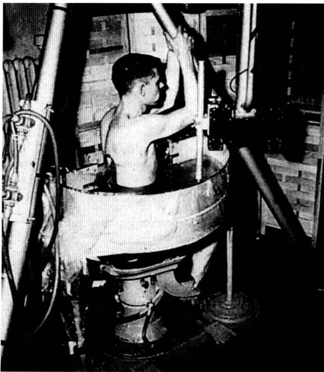
Figure 1-1 One of the early ultrasound scanning systems utilized a B-52 gun turret tank with the transducer carriage moved in a 360-degree path around the patient.
