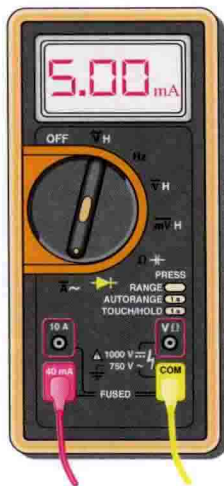
(a) Meter with yellow lead going to protoboard and red lead going to the positive terminal of the 25 V power supply.
