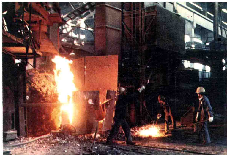
萍乡钢铁厂炼钢工在转炉前取样
