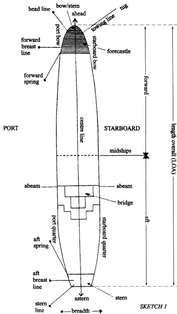
Ship's particulars refer to ship's name, call sign, kind of ship, length overall (LOA), breadth, deadweight, cargo hold capacity, draft, main engine, horse power, etc.
