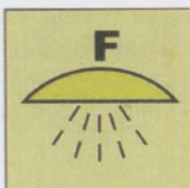
由泡沫灭火系统保护的处所 Space Protected by Foam Fire Extinguishing System
