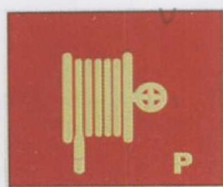
消防软管和喷嘴(干粉) Fire Hose and Nozzle(Powder)
