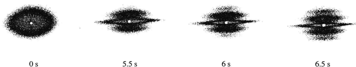
Figure 2: SALS patterns resulting from droplet break-up during flow in a dilute immiscible polymer blend (adapted from Van Hemelrijck et al. [14]).
