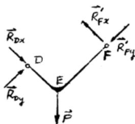
$$R_D = \sqrt{R_{Dx}^2 + R_{Dy}^2} = \sqrt{\frac{29}{32}} P$$
