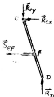
$$\Sigma F_y = 0: \quad R_{cy} = R_D = \frac{b+x}{4b} P \quad (3)$$
