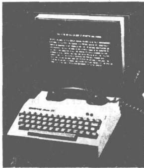
Acoustic coupler (Courtesy Digi-Log Systems, Inc.).
