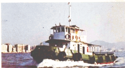
360 BHP STANDARD TUG (MODEL A) BOLLARD PULL 6.5 TONS 360匹馬力標準拖輪 (A型) 拖力6.5噸
