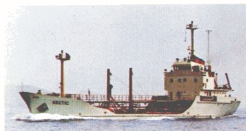
1000 DWT OIL TANKER (LR + 100A1) 1000噸油輪
