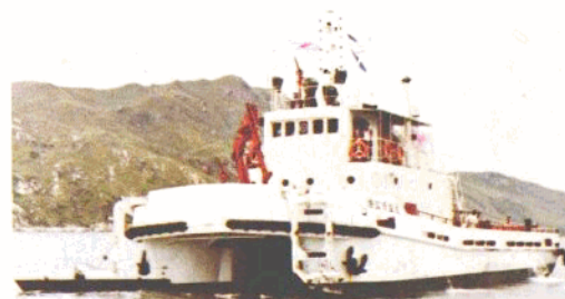
CATAMARAN TYPE OIL SKIMMER SKIMMING CAPACITY 60 CU.M/HR 雙體式掃油船回收浮油總量60立方米/小時
