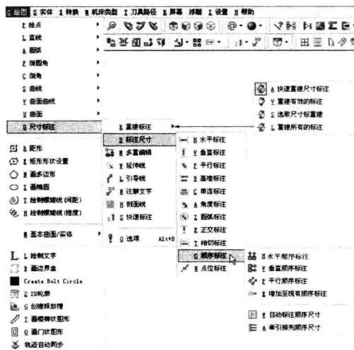
图 1-4 “绘图”|“尺寸标注”级联菜单
