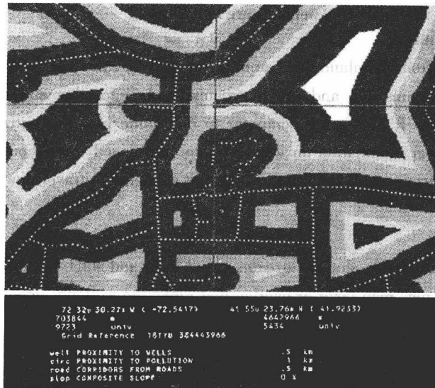
Fig. 1.23 A crosshair pointer (top) can be used to point at a location stored in a GIS. The bottom illustration depicts a computer screen containing the kind of information stored about the location—for example, the latitude, longitude, projection, coordinates, closeness to wells, sources of production, roads, and slopes of land
