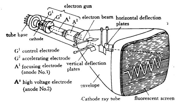
tive to any forces which act on it. When the beam of electrons strikes the front of the cathode ray tube it activates a phosphor—a material which converts electronic energy into the light which shows through the glass.
