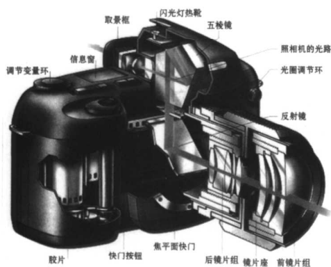
35mm单镜头反光相机剖面图 (New book of photography)
