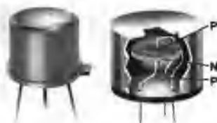
Figure 1-7 Transistor and its internal structure
