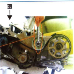
旋松此螺栓以便拆下正时带
