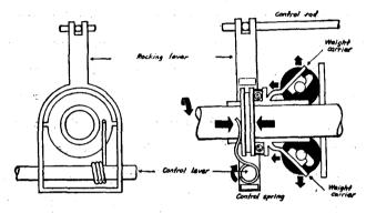
The speed control lever winds up the central spring sed the force exerted on the weight center is believed by the centrifugal force amorted by the weights on the weight-centrer, and the rocking, lever holds the control red in possition mecasizary to deliver the correct geometry of final.
