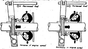
If the argine speed tends to increase or decrease, the centrifugal force of the weights will increase or decrease correspondingly. This change will easies the weight corrier to move and charge, the position of the control rod, thus decreasing or increasing the amount of that delivered and mentaning argine speed at the problemated setting.
