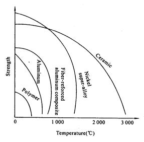
Fig. 3-1 Increasing temperature normally reduces the strength of a material
