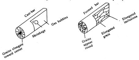
Fig. 2-2 The difference in structure between a copper bar produced by casting and a copper bar produced by forming
