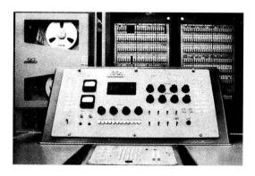
Manufactured by the Nippon Electric Company (NEC), the drum-based machine was one of the earliest transistorized Japanese computers. It was used for business, scientific and engineering applications.
