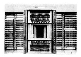
A gigantic computerized air defense system, SAGE (Semi-Automatic Ground Environment) was designed to help the Air Force track radar data in real time<sup>®</sup>. Equipped with technical advances such as modems and graphical displays, the machine weighed 300 tons and occupied one floor of a concrete blockhouse.
