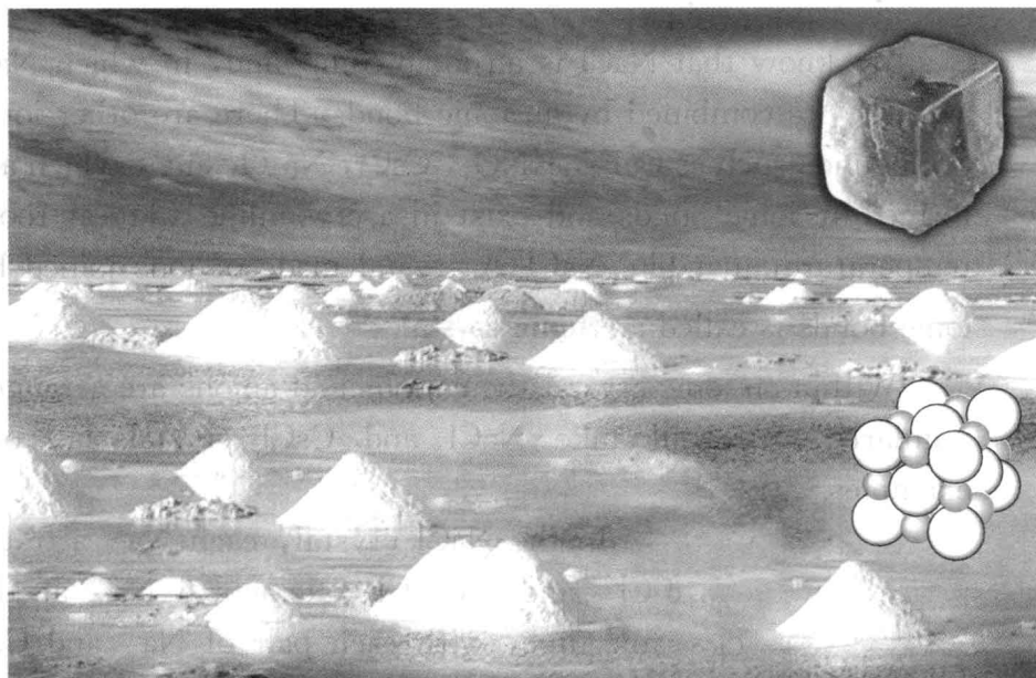
Crystal of sodium chloride and its structural model
