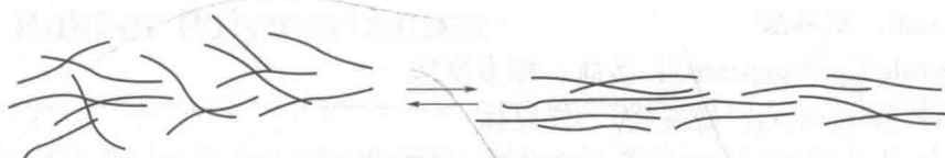
Figure 1.4 Rubbery elastomeric properties result from the stress induced uncoiling and recoiling of polymer chains
