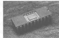
Figure 5-30 Chip mounted onto a chip carrier
