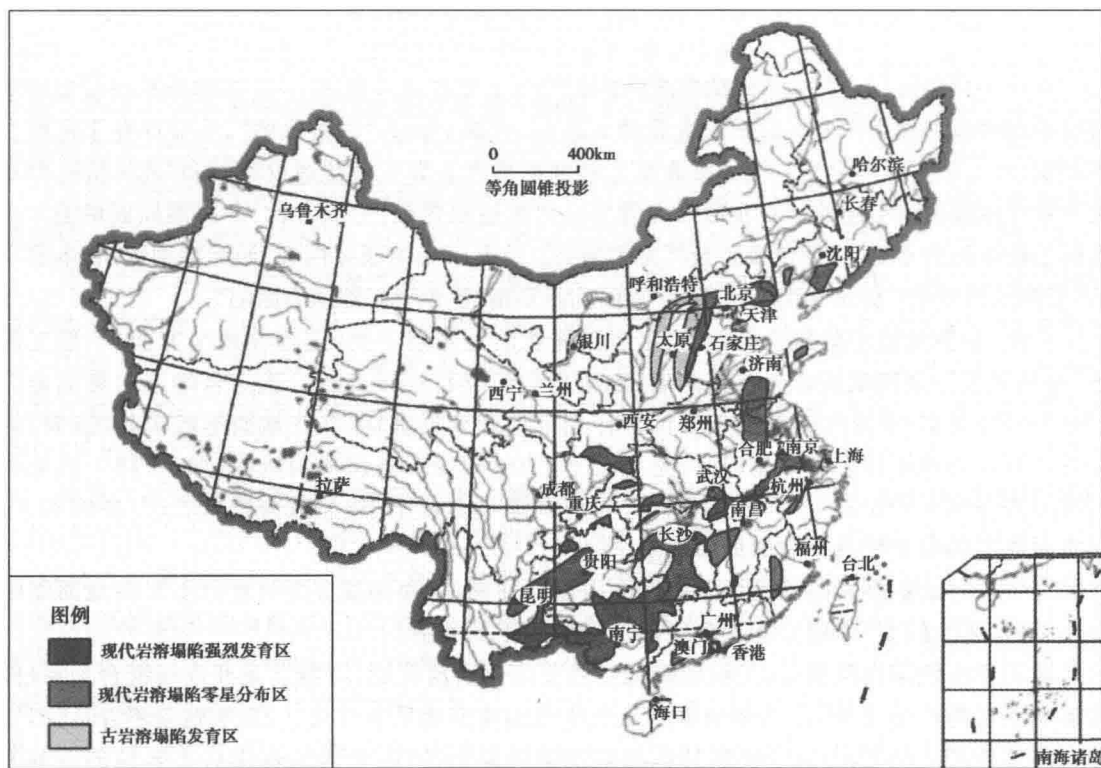
图 1-1 中国岩溶地面塌陷灾害发育区分布图(李瑞敏等, 2007) Fig. 1-1 The distribution map of karst ground collapse hazard areas in China
