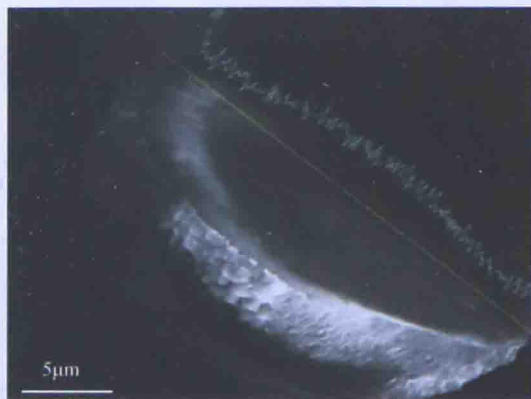
(a) (\text{Ni}_{0.25}\text{Mn}_{0.75})\text{CO}_3 断面 SEM 图
