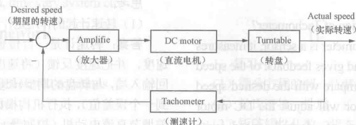
Figure 1.7 Closed-loop control of the speed of turntable 图 1.7 转盘转速的闭环控制
