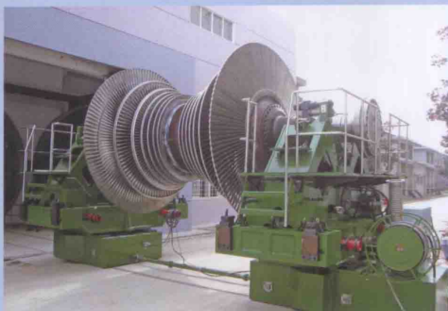
A turbine Rotor waiting for high-speed balancing
