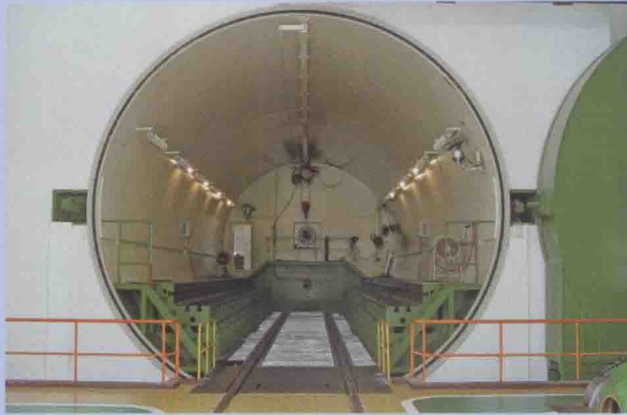
The explosion-proof vacuum cylindrical body
