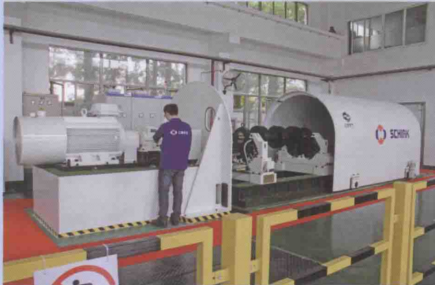
4.5t high-speed balancing and overspeed test chamber
