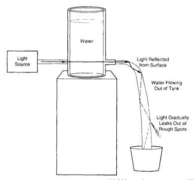
Light beam becomes more diffuse as it passes down the water jet, because turbulence breaks up surface.
