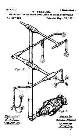
FIGURE 1.1 Wheeler's vision of piping light (U.S. Patent 247,229).
