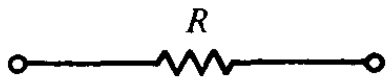
Fig. 1.12 Circuit symbol for a resistor.
