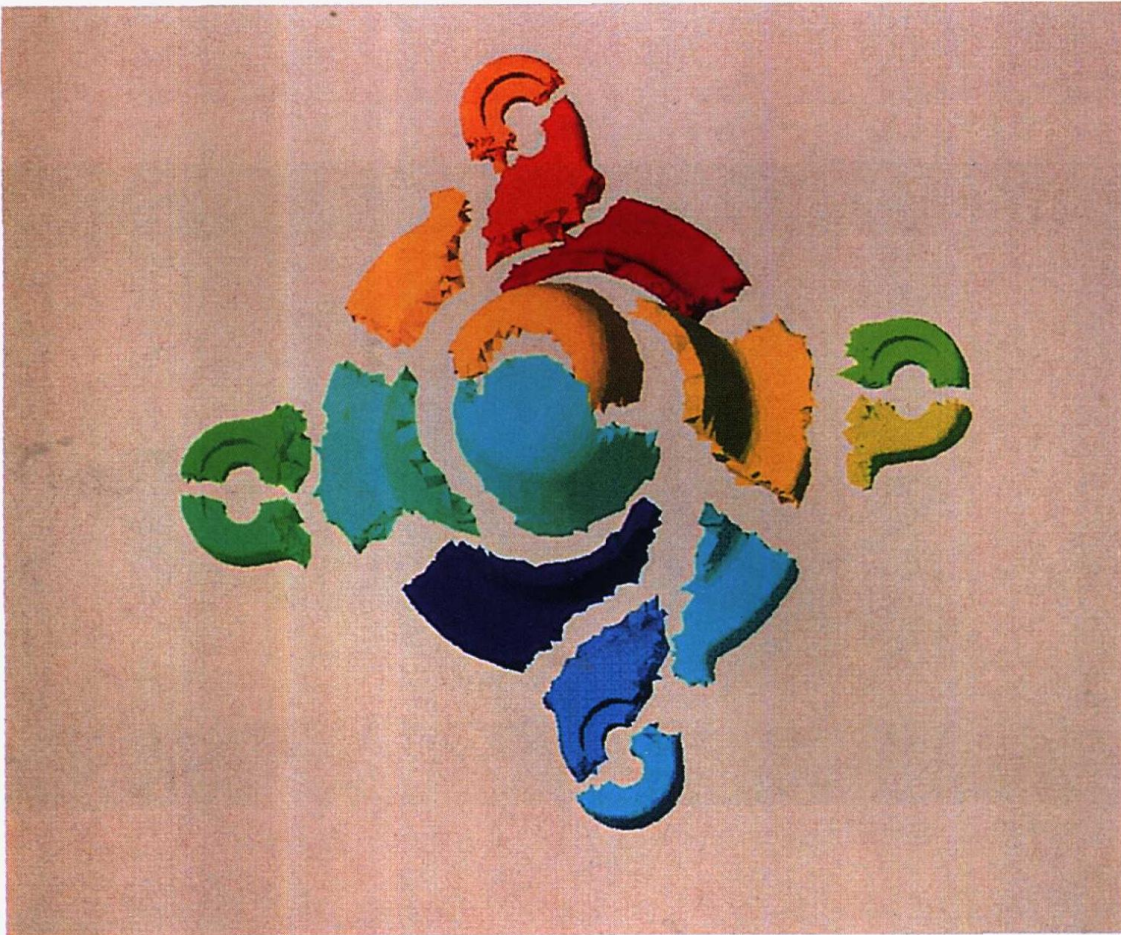
Plate 2 The spectral bisection partitioning algorithm applied to a finite element mesh generated for an assembly part. Image courtesy of Z. Johan.
