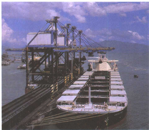
Fig. 14.4 A coal ship at the Castle Peak power station. This ship has enough coal for 5 days. About 10 000 000 tonnes are burned in a year.
