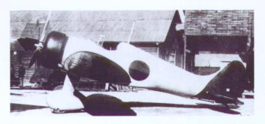
Mitsubishi A5M4 fighter: a single-seat plane made by Japan Mitsubishi Industrial Company in 1939; length: 7.56m; wingspan: 11.00m; height: 3.27m; powered with Nakajima air-cooled engine with 9 cylinders; horsepower: 785; overall weight: 1671kg; maximum speed: 434km/h; ceiling: 9800m; range: 1200km; armament: two 7.7mm-caliber machineguns, 60kg bombs.
