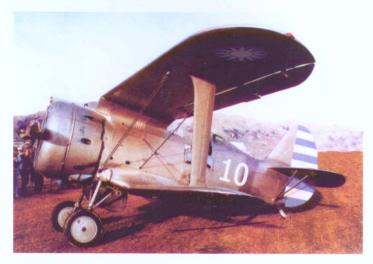
Polikarpov I-15 fighter: a single-seat plane made by Soviet Union National Aviation Industrial Company in 1934; length: 6.10m; wingspan: 9.75m; height 2.92m; powered with M25 air-cooled radial engine with 9 cylinders; horsepower: 700; overall weight: 1370kg; maximum speed: 368km/h; ceiling: 9800m; range: 500km; armament: 4 machineguns.
