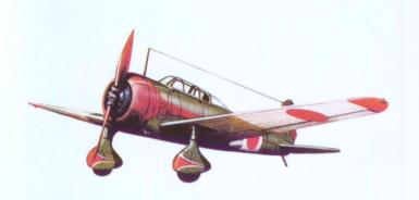
"Type 97" Nakajima Ki-27b land-based fighter: single-seat plane made by Japan Nakajima Plane Company in 1939; length: 7.53m; wingspan: 11.31m; height: 3.25m; powered with Nakajima air-cooled engine with 9 cylinders; horsepower: 710; overall weight: 1790kg; maximum speed: 470km/h; ceiling: 12365m; range: 1710km; armament: two 7.7mm-caliber machineguns, 100kg bombs.
