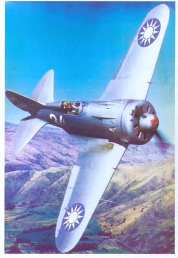
Polikarpov I-16 fighter: a single-seat plane made by Soviet Union National Aviation Industrial Company in 1937: length: 6.07m; wingspan: 9.00m; height: 2.56m; powered with M25 air-cooled radial engine with 9 cylinders; horsepower: 775; overall weight: 2054kg; maximum speed: 464km/h; ceiling: 9000m; range: 800km; armament: 4 machineguns.
