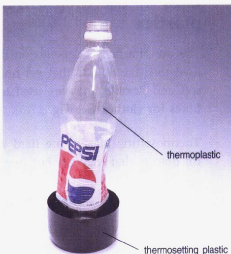
Fig. 17.4 Heat softens a thermoplastic but not a thermosetting plastic.
