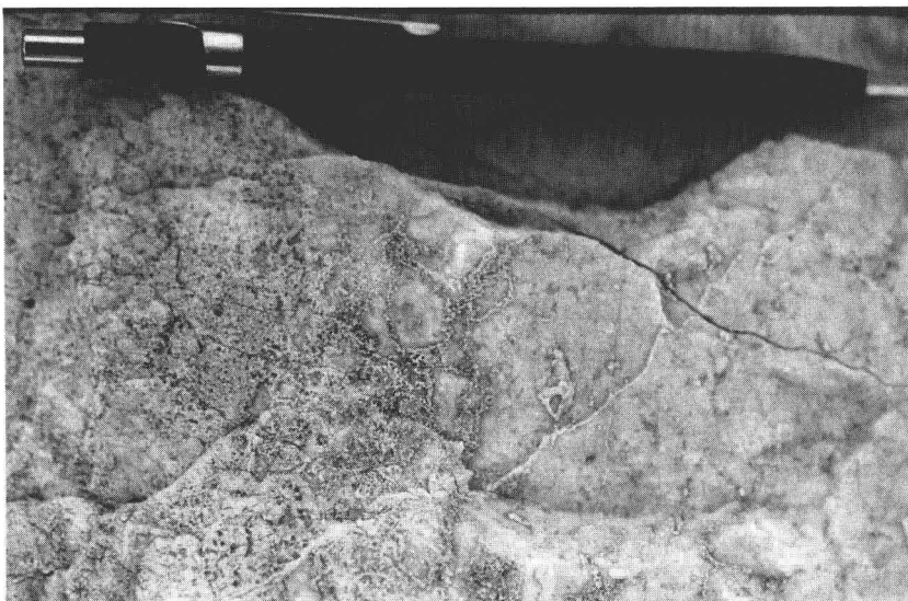
Figure 2.5. The weathered face of a partially dolomitized calcite rock in which veinlets of dolomite produced along fluid pathways stand out in relief in a dense, fine tracery on the left and along a crack on the right. (Photograph courtesy of Dr. E. N. Wilson.)
