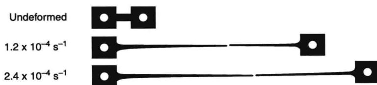
1.1 SP titanium alloy (IMI550) showing high elongations.
