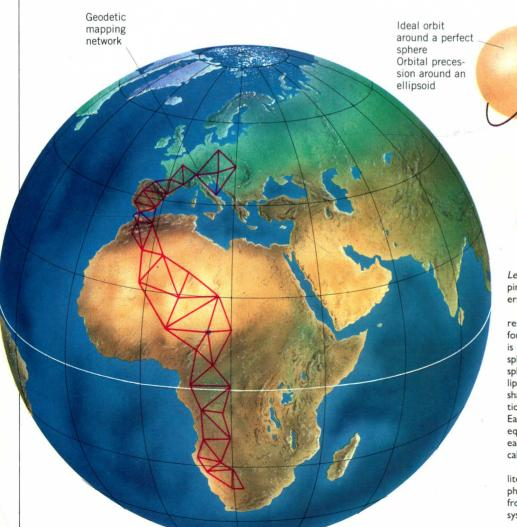
Left: The globe, with a network of geodetic mapping triangles stretching from South Africa to Eastern Europe.
