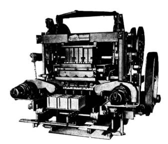
CONCRETE block-making machine, circa 1939.
