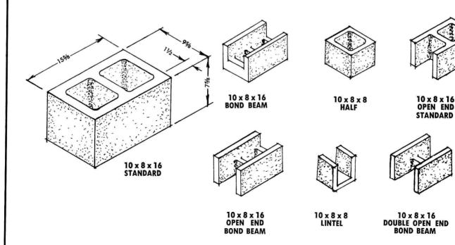
Note: Channels shown for bond beams are not to scale.
